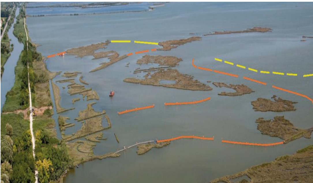
Figure 3. Aerial view of the project area with indication of the location of the morphological structures of the first section (in orange) and second section (in yellow).
